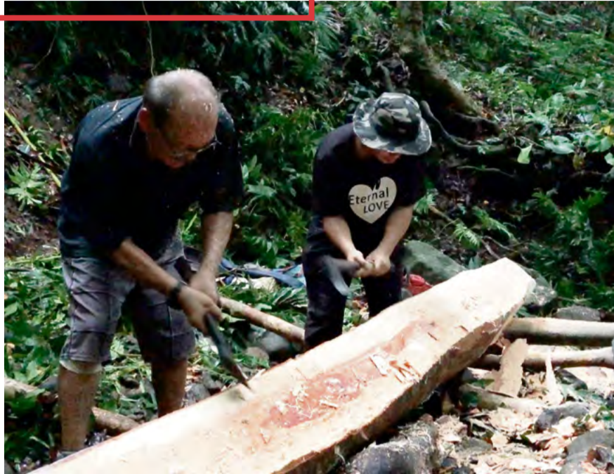
Fig. 1 (above): Carving out a plank. (Photo courtesy of Si Rapongan, 2020)
