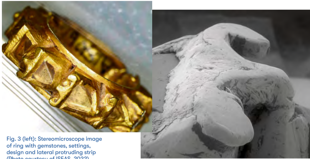
Fig. 4 (right): SEM image showing layers of gold foil with 'crown' design fused onto gemstone setting (Photo courtesy of ISEAS, 2022)
