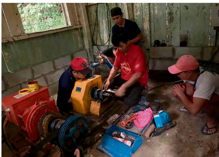
Fig. 4 (right): Indigenous community operators conducting repairs of a micro-hydro turbine at Kampung Terian Penampang, Sabah. (Photo courtesy of TONIBUNG, 2020)
