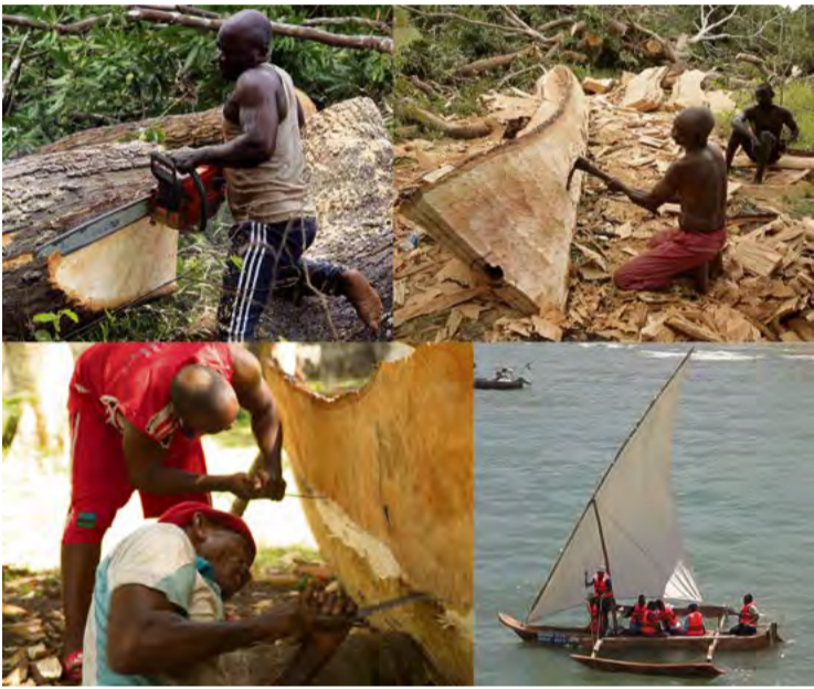
Fig. 6 (right): (right, clockwise): Mzee Alalae builds a ngalawa : rough-shaping the mango tree; shaping the hull with an adze; attaching an extension plank; the finished vessel under sail. (Photos courtesy of Bahari Yetu Urithi Wetu Project, 2021)
