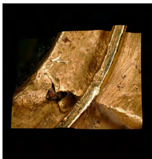
Fig. 5: 3D digital microscope image of lateral protruding strip (Photo courtesy of ISEAS, 2022)
